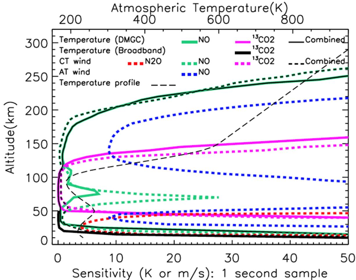
**Figure 10. Error estimates for a 3-channel DWTS instrument. See Gordley 2011**
