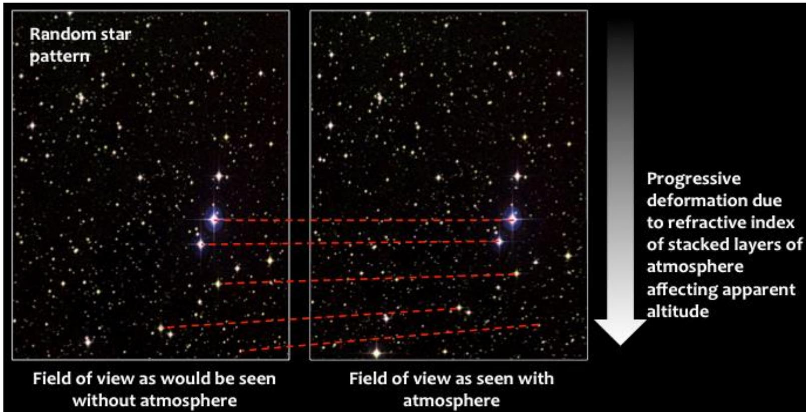
Figure 7. Refraction profiles can be derived from occulting star fields by horizontally integrating the images, then measuring the contraction of the image as a function of angle. **Tstar** is based on this concept.
