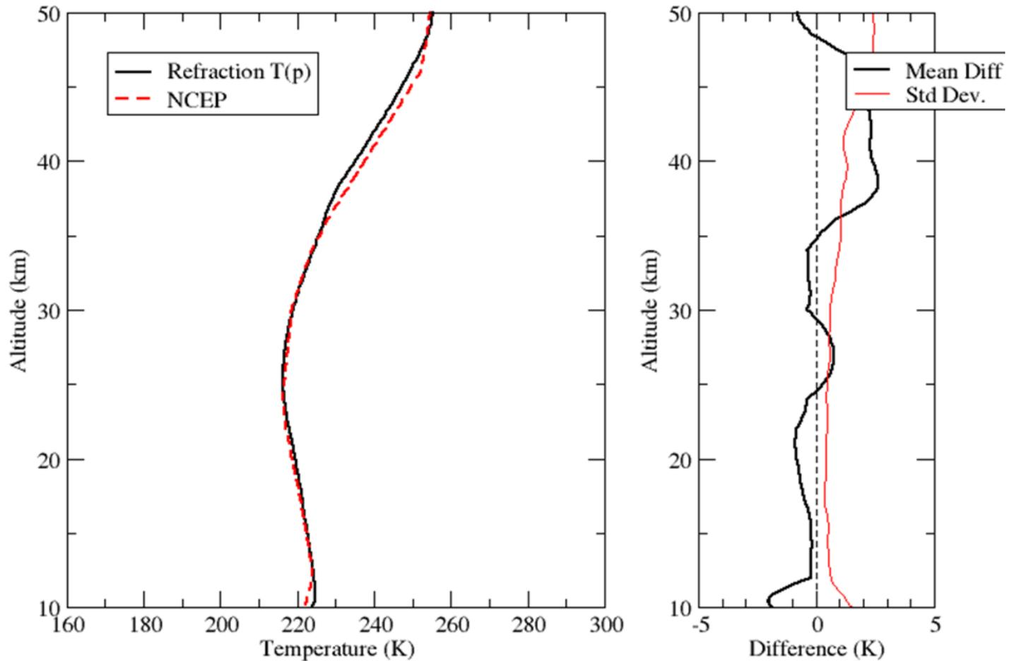
**Figure 6.** Typical statistical accuracy of temperature retrievals from the inversion of SOFIE refraction profile measurements.
