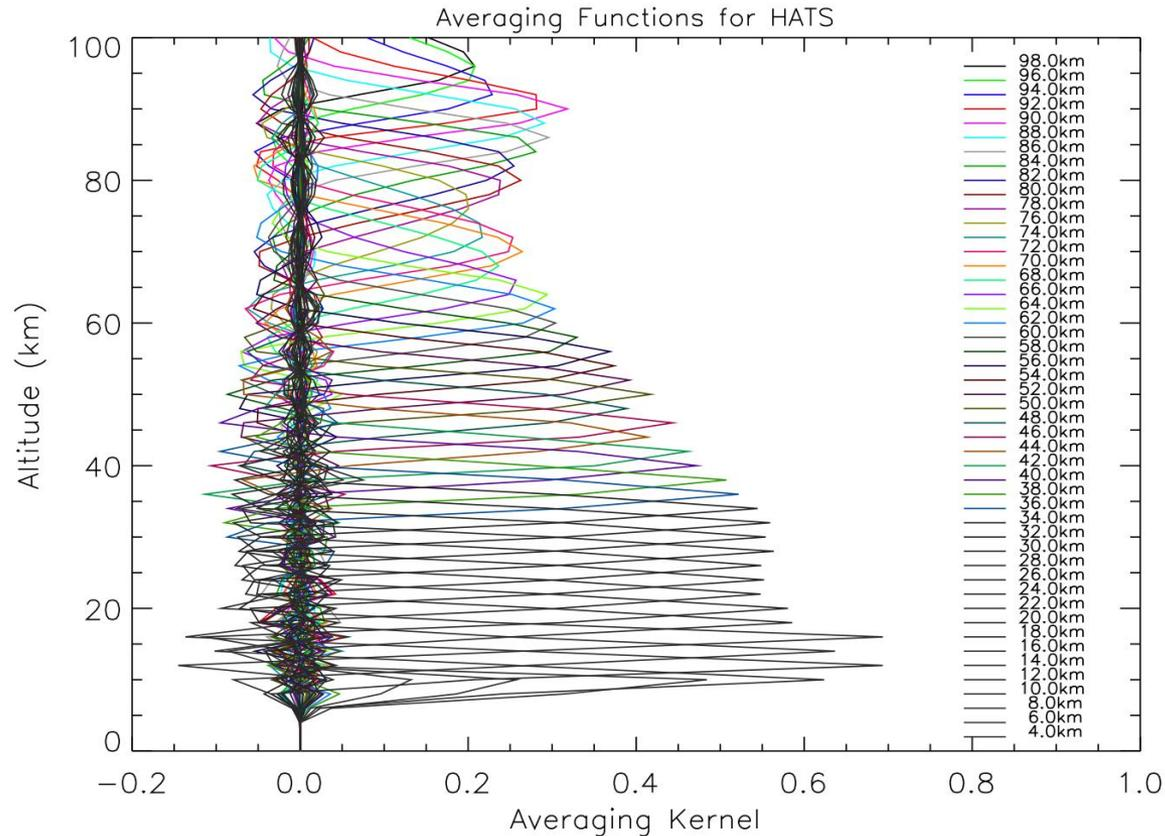
**Figure 11. Averaging kernels possible with a 7-channel DSGF instrument called **HATS**. These were created with a variety of  $\frac{1}{2}$  % filters placed throughout the spectral region shown in figure 12.**
