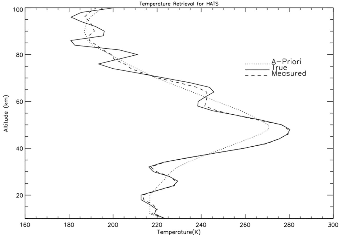
**Figure 13.** Typical **HATS** temperature retrieval using an optimal estimation approach following Rogers. The a priori is the limb T retrieval supplied by the **LCER** measurements.
