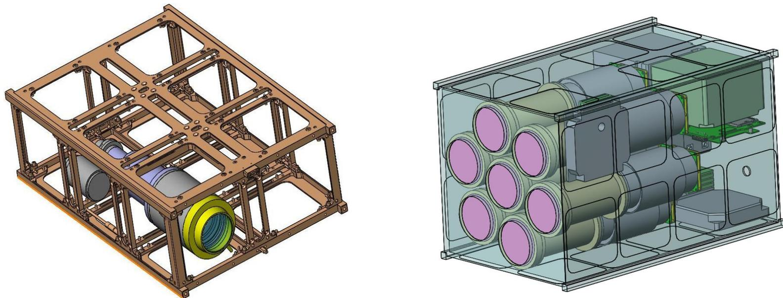
Figure 8. Every instrument in the CUAD system is a simple small imaging instrument like that depicted on left, with or without a gas cell in front of the aperture. The instrument concept on the right is for a 7-channel downward looking DSGF instrument we call **HATS** (High altitude thermal sounder (a 16 U design)).
