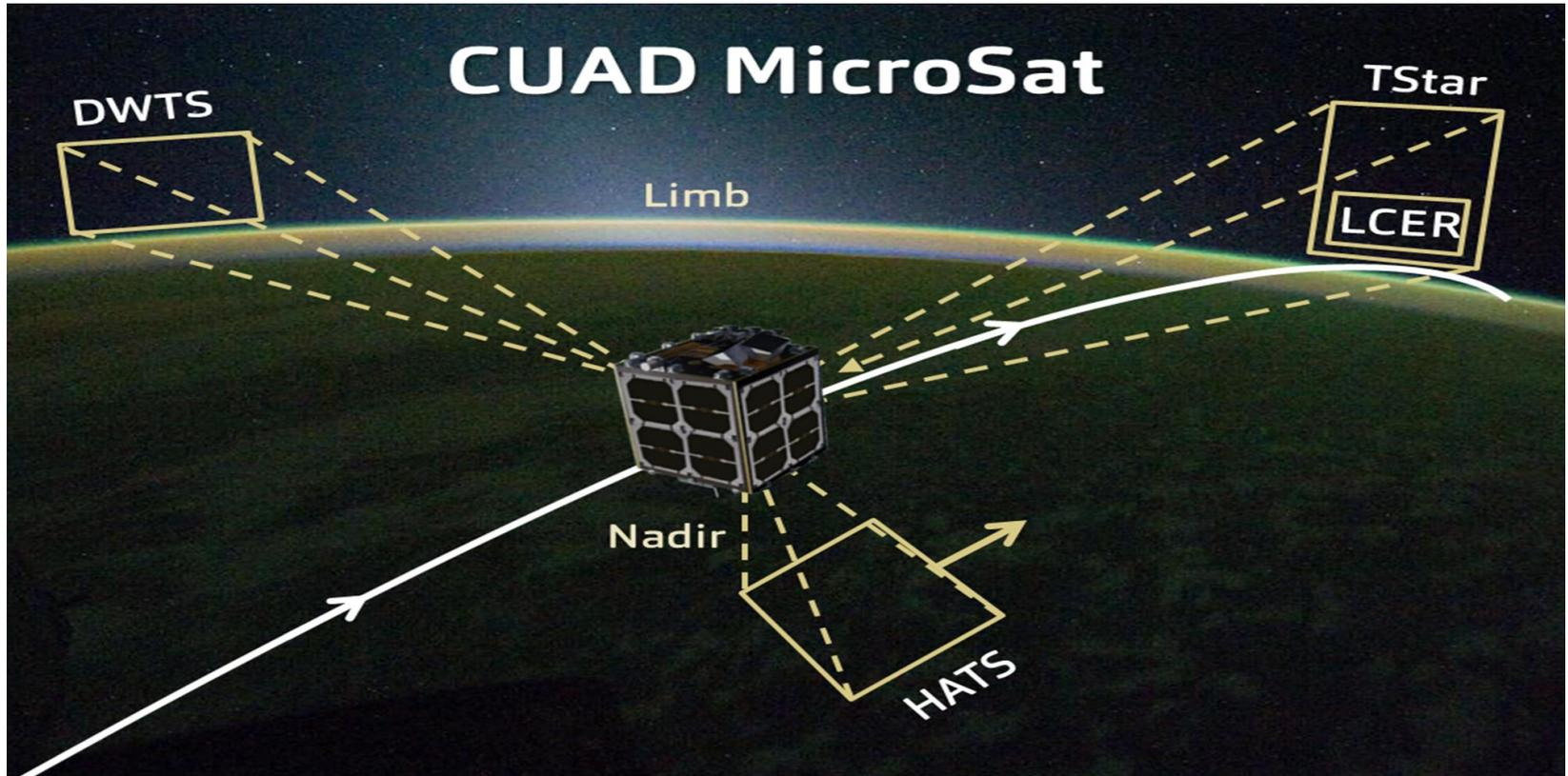
**Figure 3.** Viewing geometry of the 4 static imagers employed by the CUAD (Constellation for Upper Atmosphere Dynamics) system. The system requires no onboard scanning or calibration system
