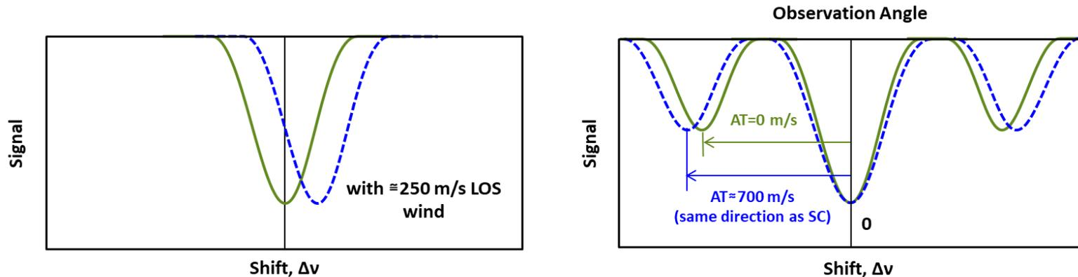
Figure 9. Example of the signal from a **DWTS** instrument. The left depicts an along-sight wind effect. The right depicts an along-track wind effect for a gas with splitting from lambda doubling (in this case nitric oxide). Temperature can also be inferred from the width of the signal dip feature. See Gordley 2011.
