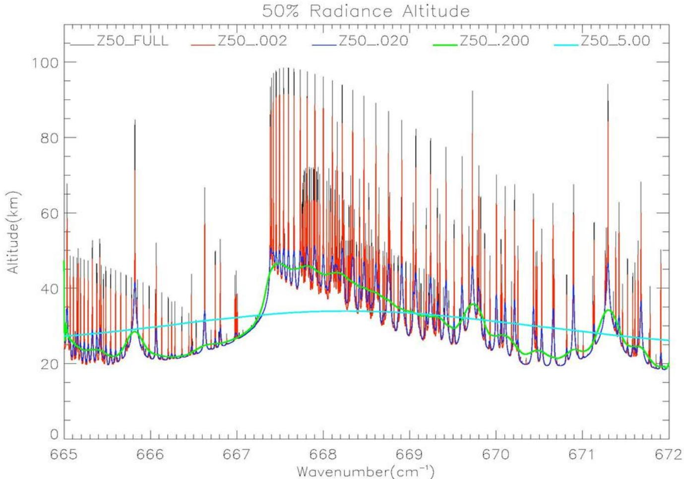
**Figure 12.** Mean altitude of emission measured with instruments of various spectral resolution. Demonstrates altitude information to 100km is possible.
