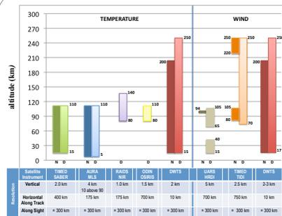
Figure 2. DWTS will dramatically improve the altitude coverage and along-track resolution of wind speed and temperature, both day (D) and night (N), compared to other past and current instruments.
