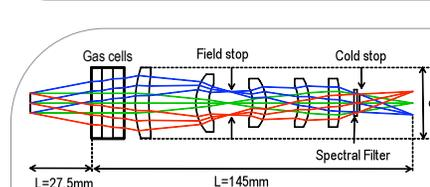
Figure 6. DWTS can be implemented with a simple refractive design, providing good stray-light rejection in a compact package, reimaging to the cold stop. Gas cells are in front of the optics to allow a single low-cost optical assembly. Fold mirrors in front of entrance aperture turn the beam to the desired limb angle relative to the optical train configuration for Nanoracks.
