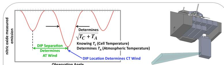
Figure 3. Emission observed (measured) from one limb location as it passes through the DWTS FOV and filtered by the gas cell. Also illustrated is the analysis used to determine temperature and wind. Example is for nitric oxide emission, which produces the half dips (side lobes) due to lambda doubling of line transitions.
