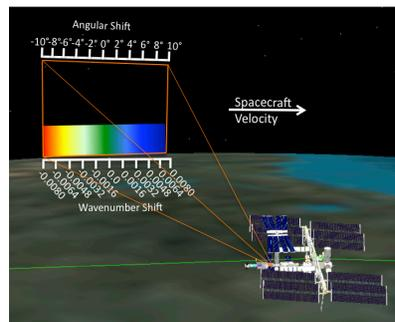
Figure 1. The DWTS instrument will view to the port side of the ISS and view the Earth's limb with a 20° horizontal and 10° vertical FOV.
